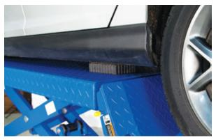
Composite polymer rubber adapter pads are placed on platforms for vehicle spotting.
