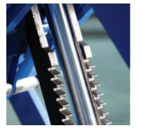
24 lock positions feature a negative rake tooth design. Locks ratchet over each other then interlock when lift is lowered to locks.
