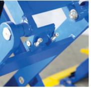
Lift dampener provides soft landing when lift is lowered to the ground.
