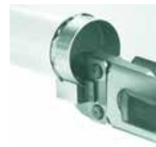
Repeat the operation until the required minimum of lugs for each diameter have been achieved.
