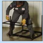
Step 1 Invert stand on concrete base with elbow mount holes to front. Hand tighten 4 legs into couplings, then torque 1/2 to 1 full turn with pipe wrench. The stand can be levelled by adjusting leg heights.
