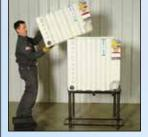
Step 3 Stack one tank on top of assembled stand with bulkhead and fill port facing outward. Align front of tank with front edge of stand (front edge has predrilled holes). Stack top tank and secure placement onto bottom tank's groves.
