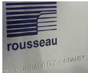
Color-filled engraving + mirror finish effect
