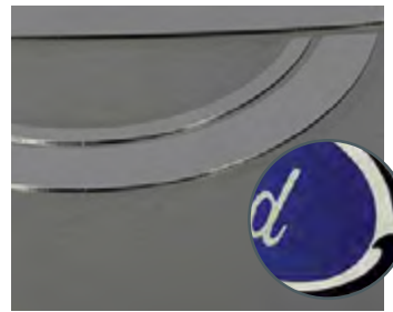
Mirror finish effect, then color-filled engraving
