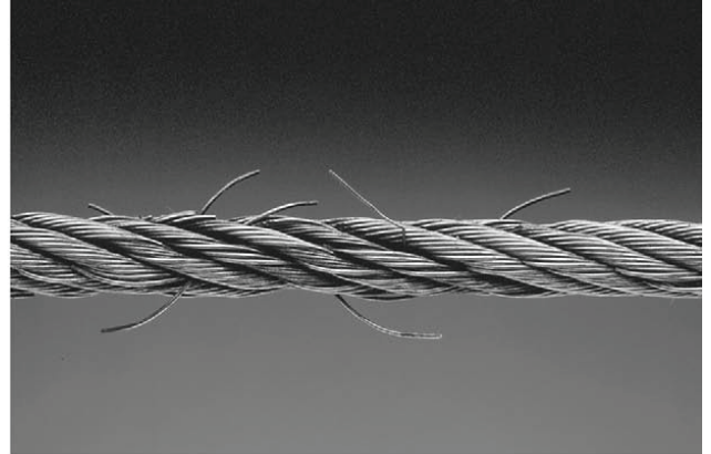
Cable With Broken Wires
